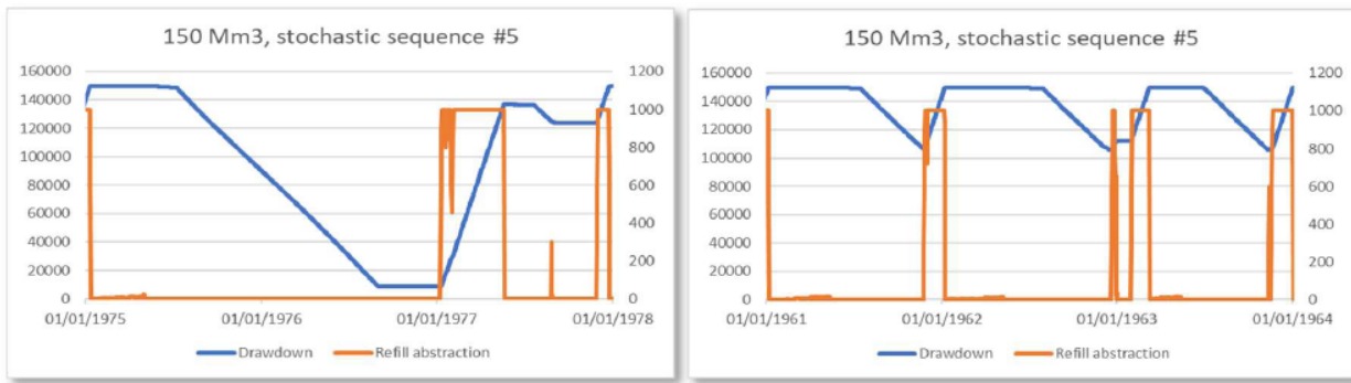
Figure 4.1 SESRO drawdown and refill – extreme drought (left) compared to standard operation (right)*
